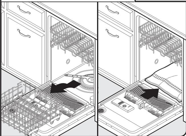
Open dishwasher door, remove lower dish rack, and place towel over pump assembly and lower spray arm of dishwasher. This will keep the screws from falling into pump area when you are securing dishwasher to countertop.
